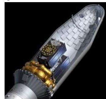
Galileo satellites 27 and 28 in their launch configuration onboard Soyuz-2 (Credit: ESA)
